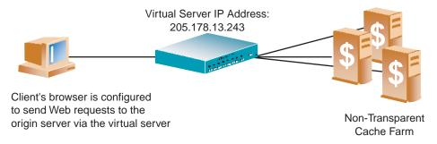
Figure 15-3 Balancing Nontransparent Caches
